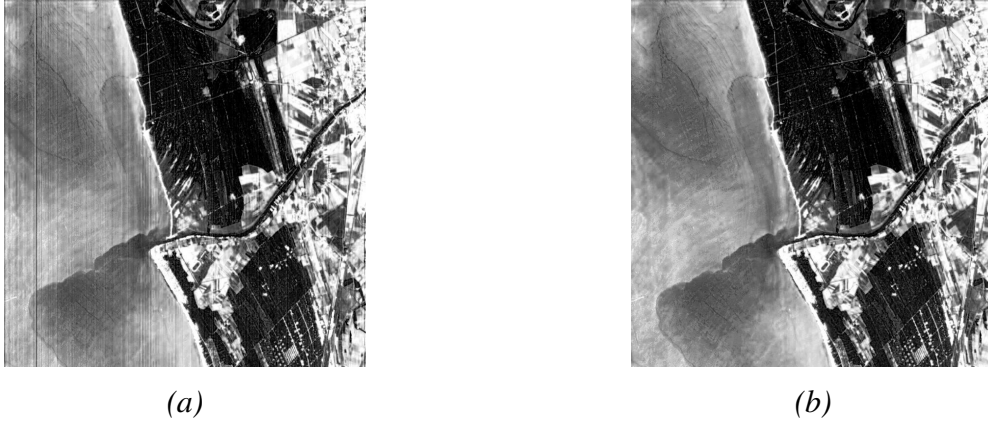
Fig. 1. CHRIS acquisition over San Rossore on August 9, 2005 (MZA = -6^\circ , FZA = 0^\circ ): (a) equalized image from the provided RCI data, (b) equalized image after removing the coherent noise.
